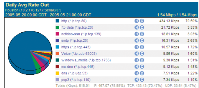
Figure 5. NetQoS ReporterAnalyzer identifies the applications, hosts, and conversations consuming bandwidth. ReporterAnalyzer may be used to quantify utilization and application volume reduction before and after a Cisco WAAS deployment.
